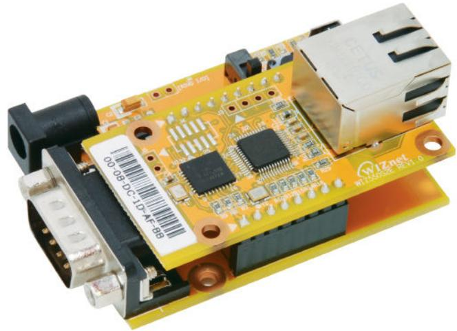
Figure 6: WIZNET serial-to-Ethernet module and development board
